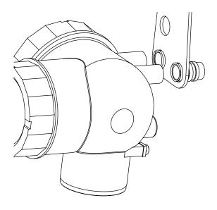
Reinstall wire routing nuts into the radar body and tighten until the flange plate is secure. (Overtightening will impact the O-rings and reduce the water resistant qualities of the radar.)
