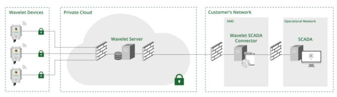
Ayyeka employs an industry-standard REST API method for data retrieval from the Ayyeka Private Cloud. In addition, Ayyeka provides three data retrieval Agents, which include DNP3, OPC-UA, and CSV, which are traditionally used for SCADA integration.
