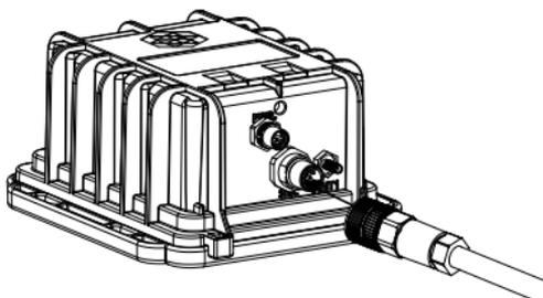
**CAUTION:** Do not turn the black plastic hood of the connector. Turning the black hood may cause the wires to disconnect, break, and/or damage the connector pins.
