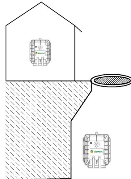
If the Wavelet is installed in an area with weak cellular signal, activate the Wavelet and place in the intended installation location with closed doors/access hatch.
