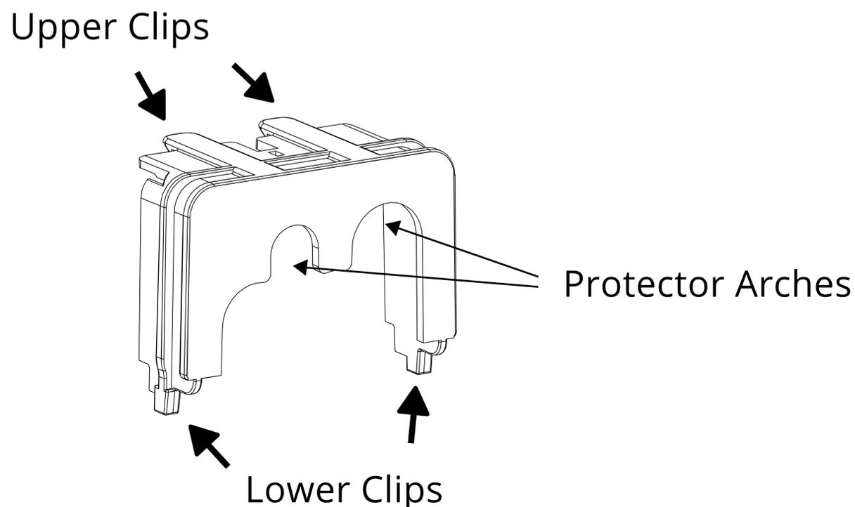
b. Snap the upper clips into place in the two grooves above the panel connector.
