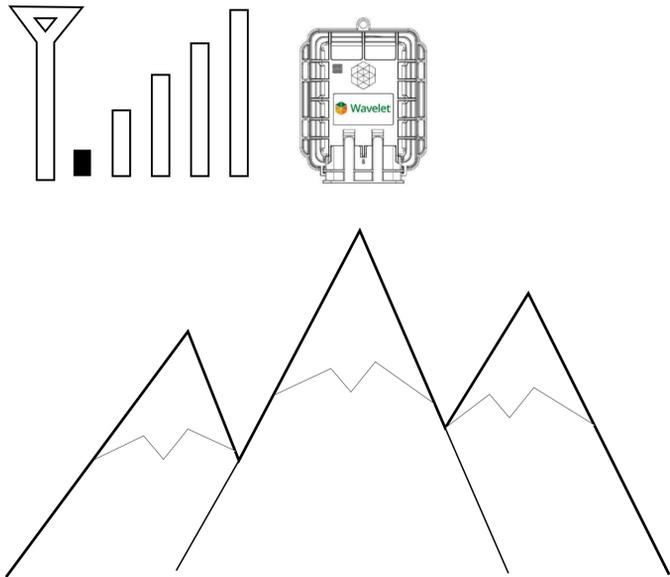
If the Wavelet is installed in an area with weak cellular signal, activate the Wavelet by using the magnetic activator.
